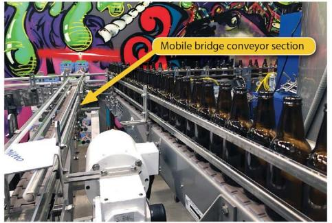
conveyors and material handling that would have to efficiently connect it all together in as little space as possible. Where would the canning line go, how could he get cans into the filler, then off the filler into labeling and packaging? How would he deal with the sudden influx of
